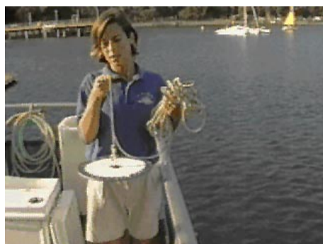
Movie 3. Determining light penetration with a Secchi disk.
